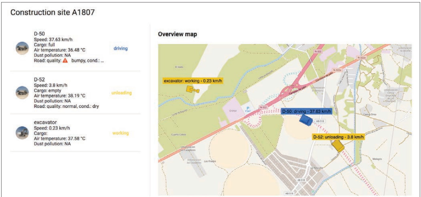
FIGURE 3. Screenshot of the user interface dashboard: a real-time view of state, locations, and activities for each tracked vehicle helps the project manager to get an overview at a glance.
